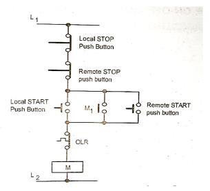
• The remote stop push buttons have been connected in series with local stop push button and the remote start-push button has been connected in parallel with local start push button. The motor can be started and stopped from any number of locations by making all the start push buttons in parallel and all the stop buttons in series.
