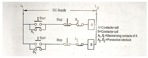
• Here our requirement is that motor A or B should run only when the other motor is in the off condition. To achieve the above condition, we have to introduce a NC (A<sub>2</sub>) of contactor A in series with the contactor coil B. Similarly, a NC (B<sub>2</sub>) of contactor B is in series with the contactor coil A. Thus, we get any one of both motors running at a time.
